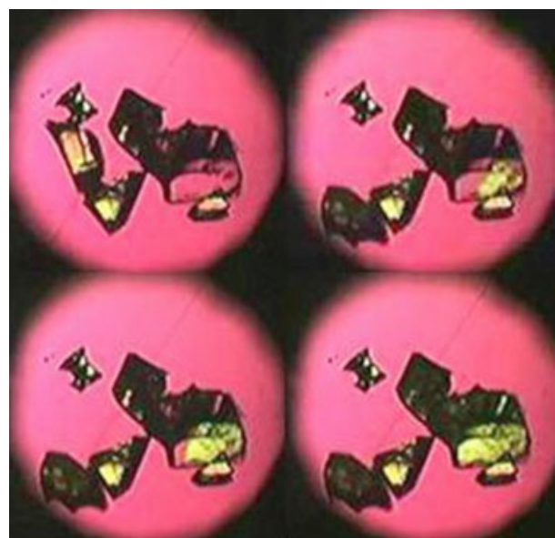
Figure 8. Thermomicroscopy of crystals of form I before the transition (top-left), when the transition started (top-right), the transition advances (bottom-left), and after transition (bottom-right).
